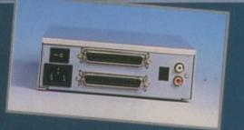
The interface simply plugs onto the 44 pin IDE connector inside the computer (still allows a 2.5" or 3.5" internal hard drive to be used as well!) and provides a connector in the blanking plate at the rear of the A1200 next to the mouse socket. This can be installed by anyone in 5 minutes!
